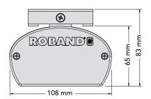
Dimensions for fabricator quartz lamps and infra-red heating assemblies (HUQ & HUE).
